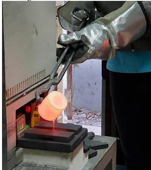
Figure 2. Pouring and casting process of molten glass into a stainless steel mold.
