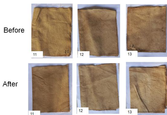
Figure 2. Cotton fabric dyed using the 40-mesh extract before and after 5 h of sunlight exposure.
