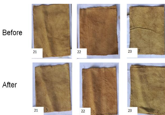
Figure 3. Cotton fabric dyed using the 60-mesh extract before and after 5 h of sunlight exposure.
