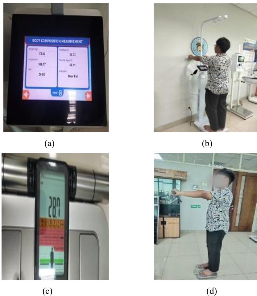
Figure 14. Conventional Body Fat Composition Testing (a, b) uses a prototype of a health kiosk, and (c, d) uses a commercial device.
