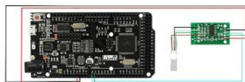
Figure 5 Schematic circuit for load cell characterization.
