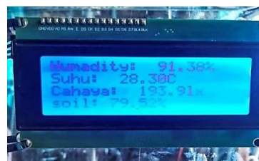
Figure 9. Results of air humidity measurements displayed on the I2C LCD.
