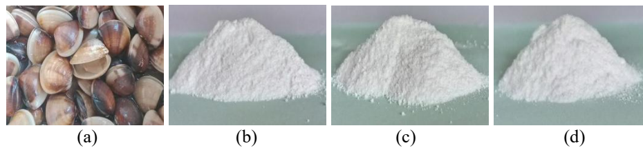
Figure 1. Raw materials (a) and HA samples with different hydrothermal times: (b) 15 h, (c) 18 h, and (d) 21 h
