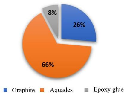
**Figure 1.** Composition of Electrode Material Mixture
