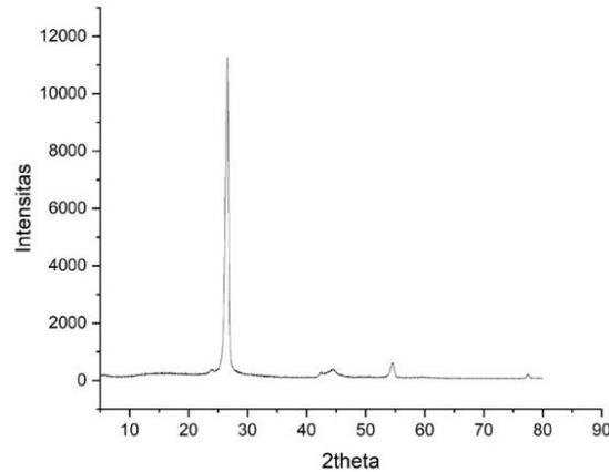
**Figure 4.** Diffraction Pattern of Graphite
