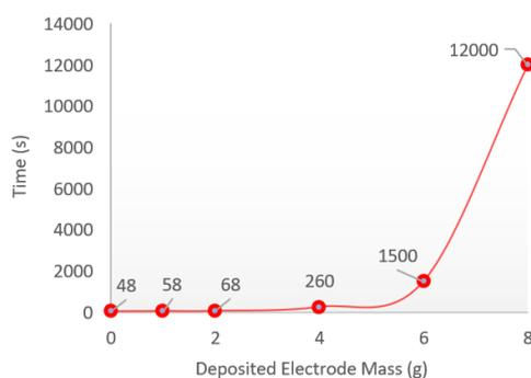
**Figure 6.** Supercapacitor Discharge Time
