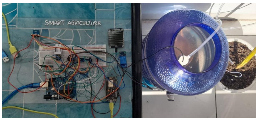
Figure 5 Implementation setup of the IoT-based automatic irrigation and environmental monitoring system for Amorphophallus muelleri (porang) plants.
