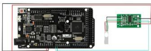
Figure 5 Schematic circuit for load cell characterization.
